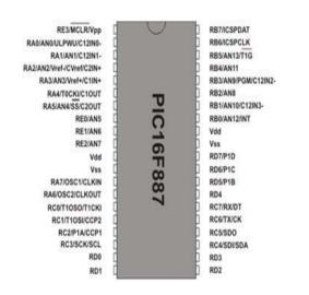
This small trick is often used because it makes the microcontroller package more compact without affecting its functionality. These various pin functions cannot be used simultaneously, but can be changed at any point during operation. The following tables refer to the PDIP 40 microcontroller.
